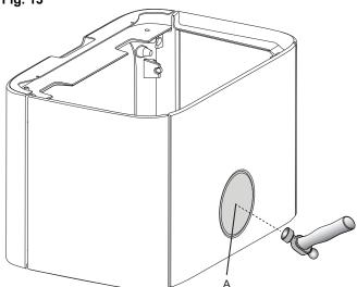
1. Place a cardboard plate on the back of the bottom plate before knocking out the cover (A) with a hammer in order to prevent the pieces from damaging something around them.
