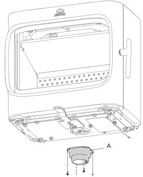
2. If external air supply is not used, the external air connector (A) can be unscrewed, if desired. Remove the four screws used for fastening the external air connector and then the connector itself. (For products with base: If necessary, you can unscrew the heat shield beneath the burn chamber in order to facilitate the dismantling of the external air connector.
