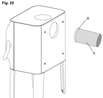
8. Place the gasket (B) on the edge of the flue pipe (A).
