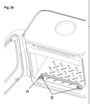
4. Fit the log retainer (A) on the knobs (B).
