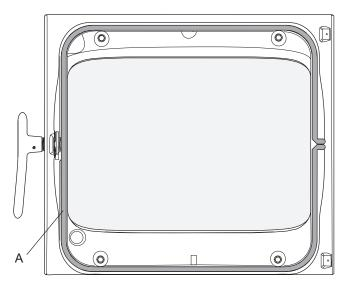
1. Remove the gasket **(A)** placed on the inside of the door, clean the gasket groove and glue on a new gasket.
