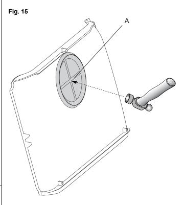
1. Place a cardboard plate on the back of the bottom plate before knocking out the cover **(A)** with a hammer in order to prevent the pieces from damaging something around them.
