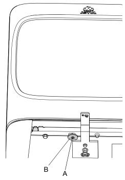
9. Unscrew the screw (A). Use the washer (B) from the bag of screws and screw it onto the burnchamber with the same screw.
