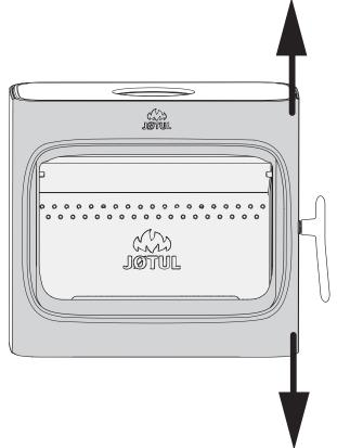
The door can be adjusted upwards or downwards slightly on the door lock side by forcing it into correct position. NB! The door cannot be fully closed when adjusting it!
