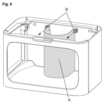
1. First remove the outside air cover (A) by unscrewing the screws (B).
