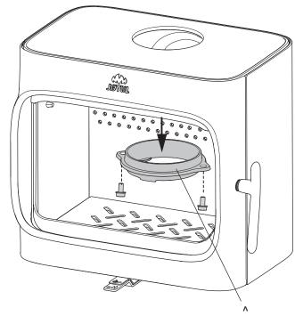
3. Unscrew the smoke outlet (A) from the top outlet.
