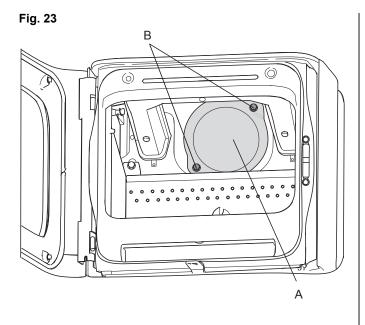
4. Unscrew the screws **(B)** and remove the cover **(A)** of the rear outlet from the inside of the burn chamber.
