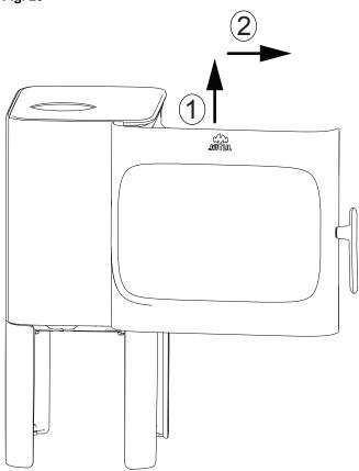
1. Open the door. Lift it up and then off the hinges.
