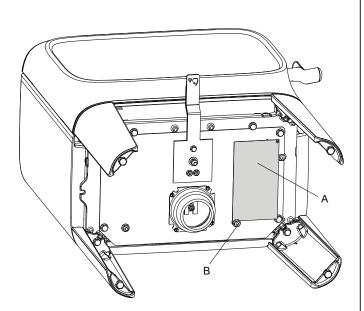
Take the approval label (A) out of the ash pan and fasten it with the nut (B), as displayed. The nut needs to be tightened only with the fingers. NB: Do not cut off the wire used for fastening the label.
