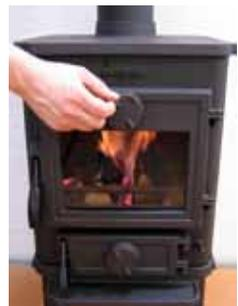
The stove door should normally be opened gently the first 2 - 3 centimetres, then you should wait until the pressure has equalised before opening the door all the way. This technique will prevent smoke from getting out, particularly when there is a poor draught.
