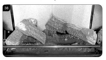
9.23 Place Log A across Log C. There is a hole on the underside of Log A which fits over the raised stud on Log C to secure in place. The small cut out on the left side of the log rests onto the log guard, see Diagram 39.
