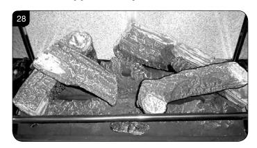
7.24 Once the logs are in place use some of the Embaglow wire wool provided and cover the ports in the burner tray with a liberal amount of fibres, in the highlighted areas shown in Diagram 29.
