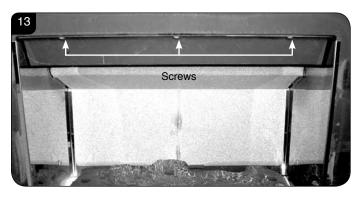
4.18 The baffle can now be removed through the front of the appliance.
