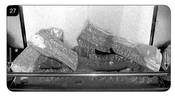
7.23 Place Log A across Log C. There is a hole on the underside of Log A which fits over the raised stud on Log C to secure in place. The small cut out on the left side of the log rests onto the log guard, see Diagram 28.
