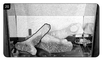
9.5 Place the small Ember at the front left of the firebox, against the rear of the log support broket to obscure the reflection of the burner screw.
