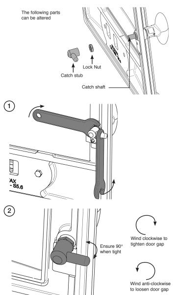
This process is the same for 1 and 2 door models, however on 2 door models the catch must sit vertical at 90° to the top of the door.
