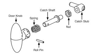
Check the door catch operation and tightness of the lock nut. Adjust if required.
