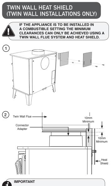
When installing the flue pipe, there must be no exposed single wall flue & a minimum 10mm expansion gap must be left between the Twin Wall flue & the top face of the Flue Collar.
