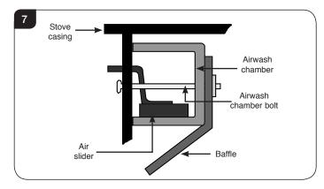
2.7 Remove the two bolts on the Airwash chamber. These are located on the inside of the stove, see Diagram 8.
