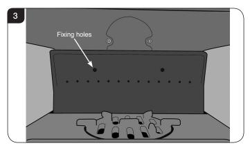
2.4 Hold the CA7560 in place and secure with the fixing bolts, see Diagram 4.
