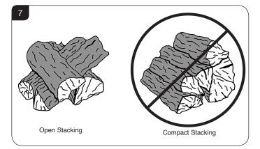
Open stacking allows oxygen to easily reach every part of the fire.
